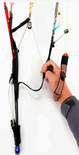
The C riser control system can be effected by pulling the toggle progressively as shown.
